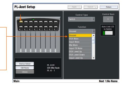
Unused LED on/off Mute Fader up/down Send level up/down FX level up/down PAFL Scene recall Custom MIDI string Talkback assign
